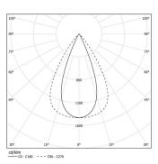
Beam angle Flood 65° Application Weight
