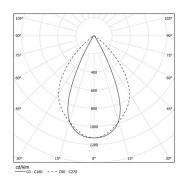
Beam angle Wide flood 80° Application Weight
