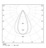
Beam angle Flood 65° Application Weight
