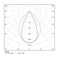
Beam angle Wide flood 80° Application Weight
