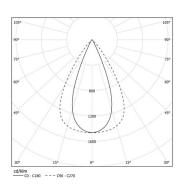
Beam angle Flood 65° Application Weight
