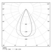
Beam angle Flood 65° Application Weight
