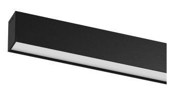
Design: Eduardo Souto de Moura Surface or pendant luminaire with housing made of aluminium profile with 25micron maximum corrosion resistance anodization with matt finish or with textured electrostatic 100% polyester paint. Frosted polycarbonate diffuser with user friendly clipping system and double fitting system: flushed or recessed.
