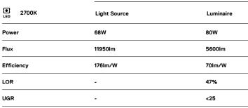
Beam angle Diffuse Application Weight 4,5Kg \_\_\_\_\_C0 - C180 \_\_\_\_\_ - C90 - C270
