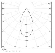
Beam angle Flood 50° Application Weight 0,8Kg
