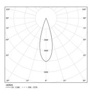
Beam angle Medium 30° Application Weight 0,8Kg
