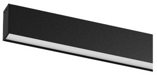
Design: Eduardo Souto de Moura Surface or pendant luminaire with housing made of aluminium profile with 25micron maximum corrosion resistance anodization with matt finish or with textured electrostatic 100% polyester paint. Frosted polycarbonate diffuser with user friendly
