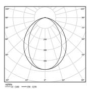
Beam angle Diffuse Application Weight 1,7Kg
