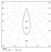
Beam angle Medium 31° Application Weight 2,4Kg
