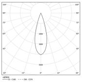
Beam angle Medium 31° Application Weight 2,4Kg
