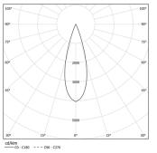
Beam angle Medium 31° Application Weight 2,4Kg
