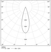
Beam angle Medium 31° Application Weight 2,4Kg
