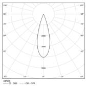
Beam angle Medium 31° Application Weight 2,4Kg
