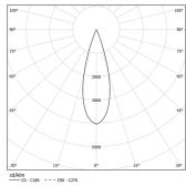
Beam angle Medium 31° Application Weight 2,4Kg
