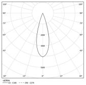
Beam angle Medium 31° Application Weight 2,4Kg
