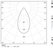
Beam angle Flood 52° Application Weight
