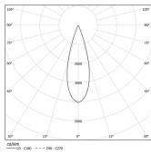
Beam angle Medium 31° Application Weight 2,4Kg
