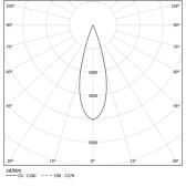
Beam angle Medium 31° Application Weight 2,4Kg
