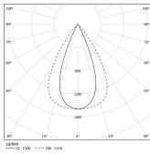
Beam angle Flood 64° Application Weight
