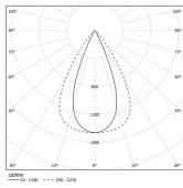
Beam angle Flood 64° Application Weight
