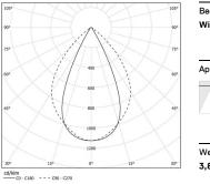
Beam angle Wide flood 76° Application Weight
