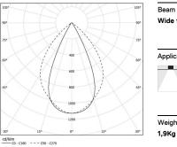
Beam angle Wide flood 76° Application Weight
