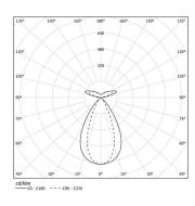
Beam angle Flood 64° / batwing
