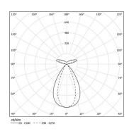
Beam angle Flood 64° / batwing
