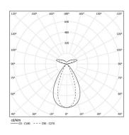
Beam angle Flood 64° / batwing
