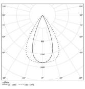
Beam angle Flood 64° Application Weight
