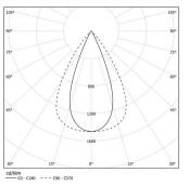
Beam angle Flood 64° Application Weight
