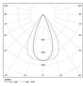
Beam angle Flood 64° Application Weight
