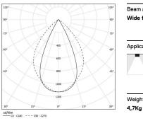
Beam angle Wide flood 76° Application Weight
