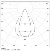
Beam angle Flood 64° Application Weight
