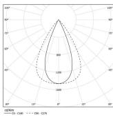
Beam angle Flood 64° Application Weight
