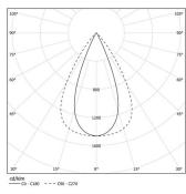
Beam angle Flood 64° Application Weight
