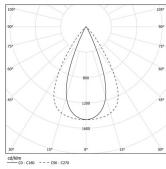
Beam angle Flood 64° Application Weight
