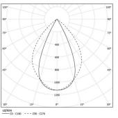
Beam angle Wide flood 76° Application Weight
