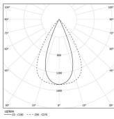
Beam angle Flood 64° Application Weight
