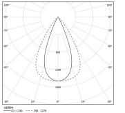
Beam angle Flood 64° Application Weight 4,7Kg
