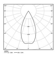
Beam angle Flood 59° Application Weight 0,64Kg
