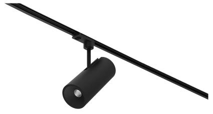
Design: O/M + Bartenbach GmbH Track-mounted spotlight with die-cast aluminium body with electrostatic 100% polyester paint finish. Spot-lens with individual complex surface rips to provide a focal light and an extremely narrow beam. Orientable by 90° horizontal rotation and 330° vertical rotation.
