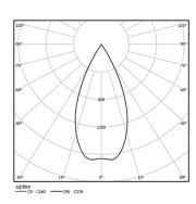
Beam angle Flood 59° Application Weight 0,64Kg
