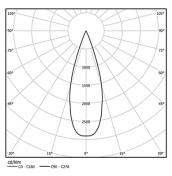
Beam angle Medium 41° Application Weight 0,64Kg
