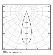
Beam angle Medium 41° Application Weight 0,64Kg
