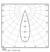
Beam angle Medium 41° Application Weight 0,64Kg
