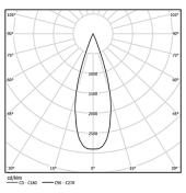
Beam angle Medium 41° Application Weight 0,64Kg
