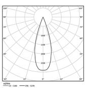
Beam angle Medium 41° Application Weight 0,64Kg
