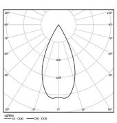
Beam angle Flood 59° Application Weight 0,64Kg
