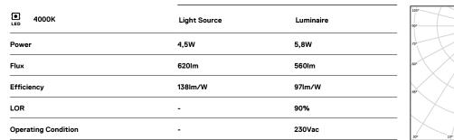
Beam angle Flood 59° Application Weight 0,64Kg
