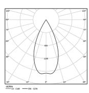
Beam angle Flood 59° Application Weight 0,64Kg
