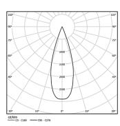
Beam angle Medium 41° Application Weight 0,64Kg
