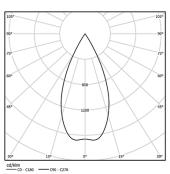
Beam angle Flood 59° Application Weight 0,64Kg
