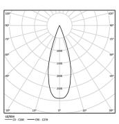
Beam angle Medium 41° Application Weight 0,64Kg
