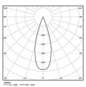
Beam angle Medium 41° Application Weight 0,64Kg
