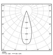
Beam angle Medium 41° Application Weight 0,64Kg
