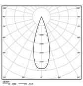
Beam angle Medium 41° Application Weight 0,64Kg
