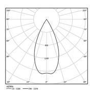
Beam angle Flood 59° Application Weight 0,64Kg
