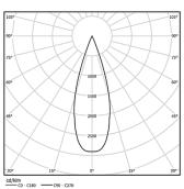
Beam angle Medium 41° Application Weight 0,64Kg
